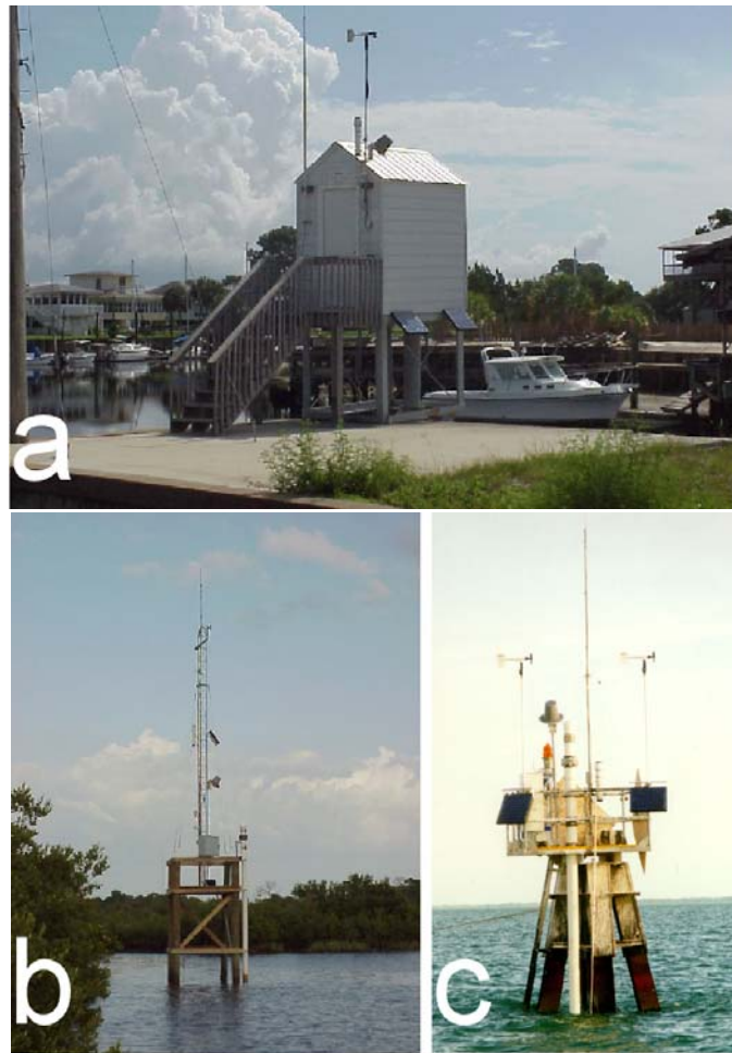
COMPS water level sites. (a) Shell Point (b) New Port Ritchey, and (c) Cape Sable sites. Aquatrak sensor (white pipe) is placed as high as possible to capture maximum surge.
